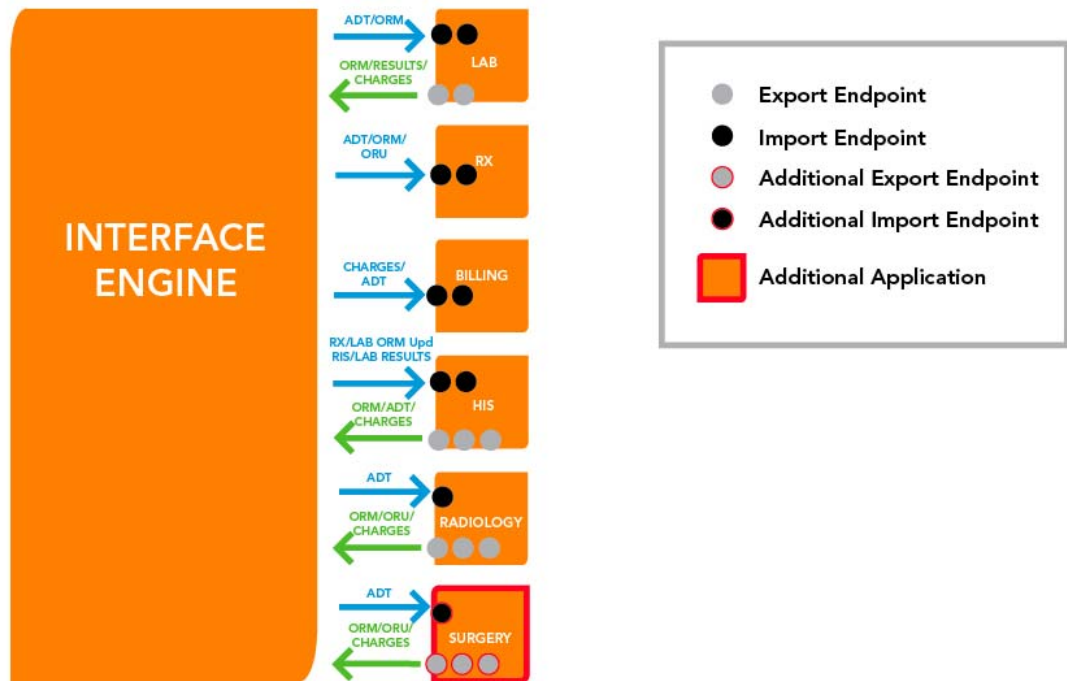
Figure 9: Adding Application in engine model Requires 4 interfaces at an approximate cost of $40K
